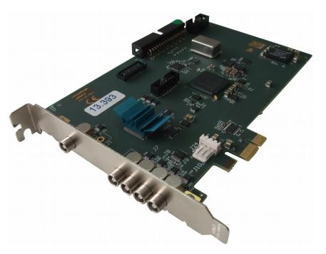
The TimeTagger4-1G-PCle is a high bandwidth, low cost common start time-to-digital converter (TDC). The timestamps of leading or trailing edges of digital pulses are recorded with a single shot time resolution of 1000 ps.
