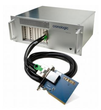
With the Ndigo Crate it is possible to use up to 5 PCle boards and 2 PCl boards with a PC. The connection of the external chassis to the PC happens over PCle2 x16 for a full duplex bandwidth of 2x 8GByte/s.
